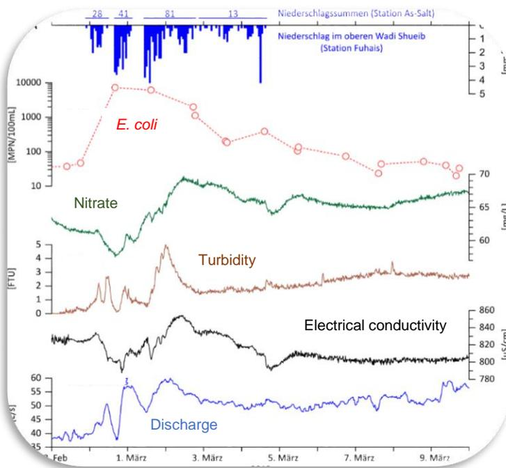
In the Wadi Shueib Catchment time series correlation analyses showed that infiltrated rain water transfers the fecal contamination in groundwater karst system quickly to the springs. This mechanism threatens the local water supply. Unfortunately, it was not feasible to monitor *E. coli* bacteria continuously by an automated measuring station. To establish a preventive protection, a parameter combination, which could indicate bacterial contamination, was developed.
