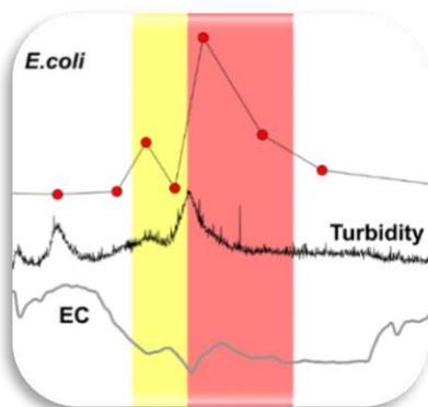
Indeed, an empirical relationship between major rain events and subsequent bacterial contamination was identified. Adding the parameters electrical conductivity and turbidity into this analysis, results in a more robust correlation. This forms the basis of our early warning system (EWS).
